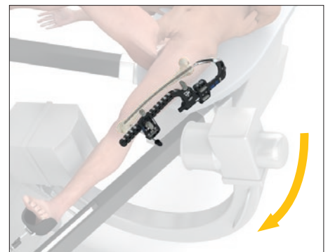
Fig. 78: Adjust C-arm down.
